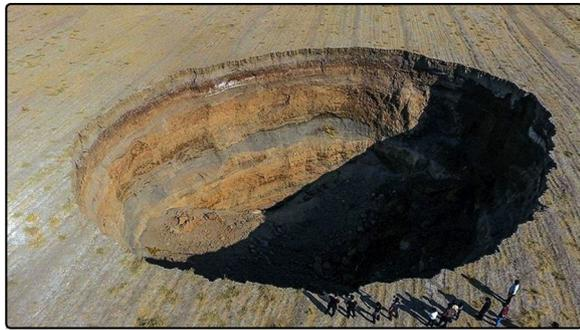
**Fig. 7** Ground subsidence phenomenon (eastern plains of Kurdistan, Dehgolan, and Qorveh), 2019
